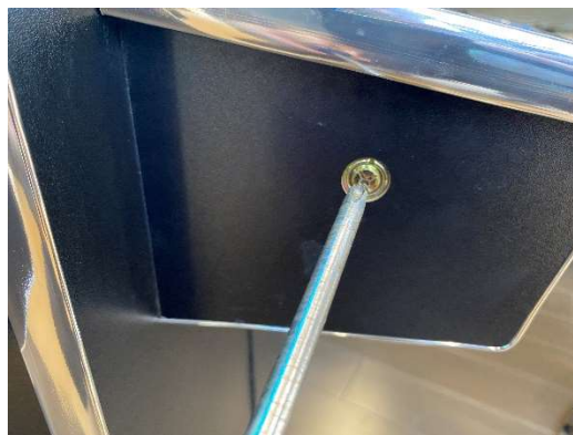
Image 14 - Set screws to remove control panel
